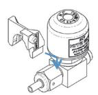
1) Mount the valve Lock Assist component.
