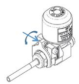
After checking the clearance A dimensions\*1, tighten the bolt at the specified torque\*1.
